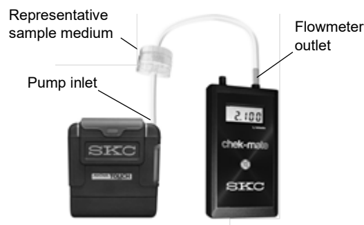
Figure 2. Medium and Low Flow Rate Verification Train (Medium Flow Pump and Flowmeter Shown)
